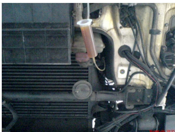
Fig. 5. ICE treatment of a BELAZ haul truck owned by Kuzbassrazrezugol Coal Company OJSC, Kedrovsky Coal Mine branch using ART compounds (Neosphere LLC). Testing Laboratory of Fuels and Lubricants, 2006
